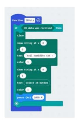
A code block that performs manual watering when the user presses the OK button. We used the preset IR control function.
