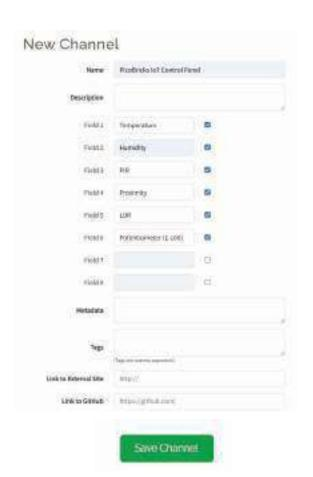
7. We have now created the necessary channel to print the data obtained from PicoBricks modules. We will use the following 'API Keys' in the code blocks we will create in MakeCode to write the data to the channel
