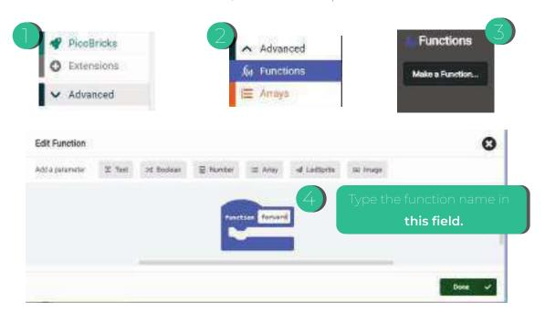
b) Let's create 5 functions named Forward, Backward, Right, Left, and Stop. Then, drag the DC Motor blocks from the "Motor" blocks in the "PicoBricks" extension into the function blocks as shown in the visual below.
