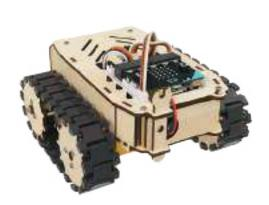
Attach the tracks for the other side by following previous assembly steps.
