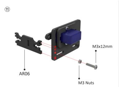
\*In order to connect the parts together properly, first insert the screw (1). then put nut inside the referenced nesting (2) then its safe to tighten screw (3).
