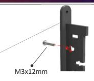
In order to connect the parts together properly, first insert the screw (1). then put nut inside the referenced nesting (2) then its safeto tighten screw (3).
